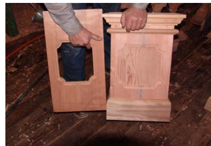
Eric shows the method he uses for creating raised panels.
